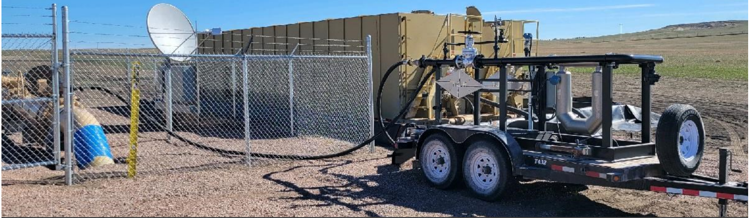
Pictured above - instrumented leak skid used for commodity withdrawal tests
